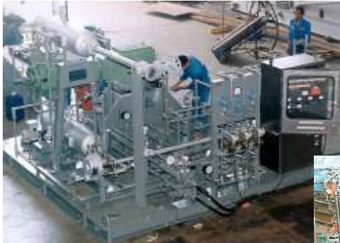
High-pressure H 2 S compressor for Shell-refinery, Port Dickson Malaysia
