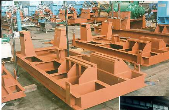
API 610 Base-frame of pumping-system for Combined-cycle Power Plant Tambak Lorok
