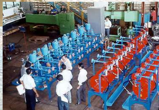
Lub-Oil Central Distribution-System for Kaltim Prima Coal Mining in Sangata
