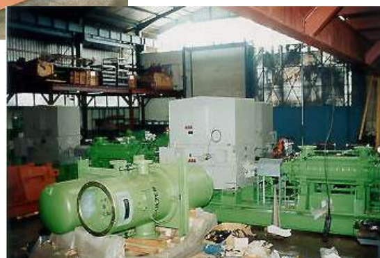
Boiler Feed Water Pump 1,8 MW for Coal-fired Power Plant Muara Tawar
